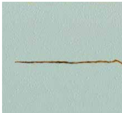
300 H SALT SPRAY TEST
